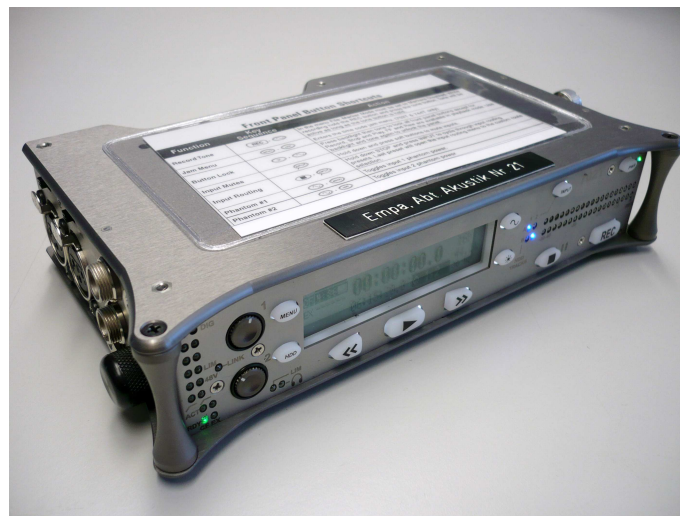
Figure 4.11: Example of a harddisk recorder as a stand-alone device.
