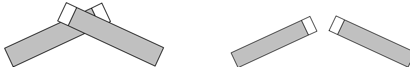
Figure 5.2: left: correct XY arrangement (sound from the left hits the left microphone firstly), right: wrong XY arrangement (sound from the left hits the right microphone firstly).
