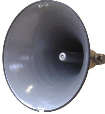
Figure 3.13: Example of a horn loudspeaker. The horn is folded to achieve a smaller overall length of the speaker.
