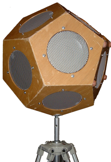
Figure 7.30: Dodecahedron loudspeaker with 12 chassis for omnidirectional sound radiation.
