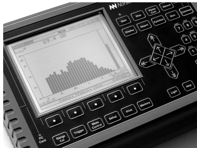
Figure 2.9: Example of a hand-held third-octave band analyzer.
