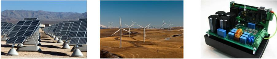
Non-synchronous generation connected via **power electronics**
