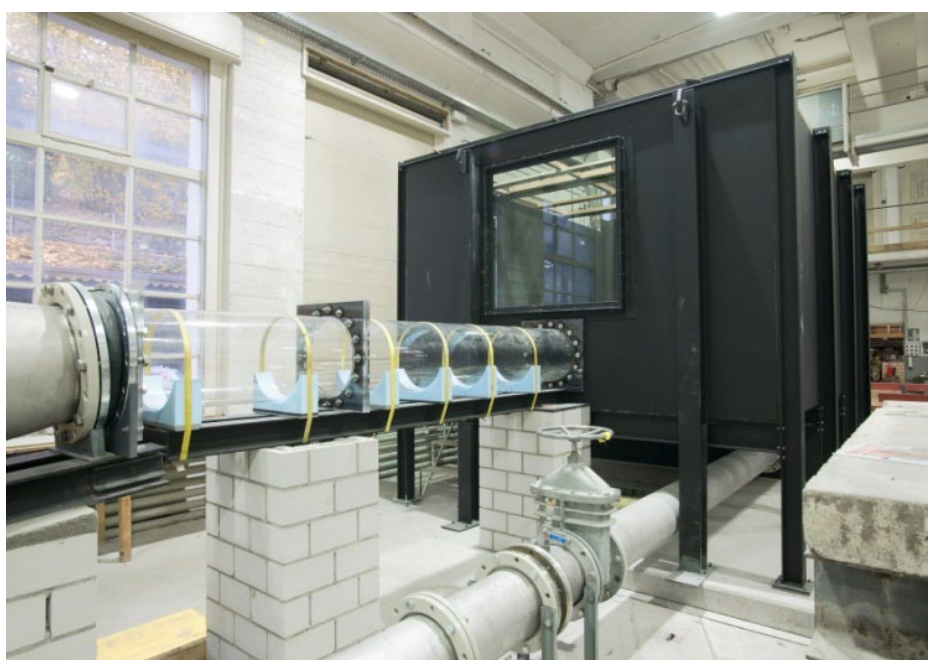
Fig. 1: Physical model with tank (black) and a horizontal outlet pipe (plexiglass, d = 0.4 m).
