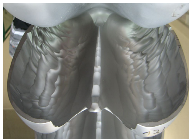
Fig. 2: Example of a Pelton runner, showing heavy damage caused by hydro-abrasive wear. The bucket splitter is no longer sharp and the bucket is “washed out” (TIWAG).
