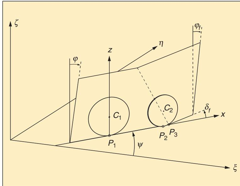
**Figure 2.** Coordinate systems. The orthogonal system  $\xi\eta\zeta$  is fixed to inertial space, and the  $\zeta$ -axis is vertical. The orthogonal system  $xyz$  has its origin at the contact point of the rear wheel with the  $\xi\eta$  plane. The  $x$  axis passes through the points  $P_1$  and  $P_3$ , while the  $z$  axis is vertical and passes through  $P_1$ .
