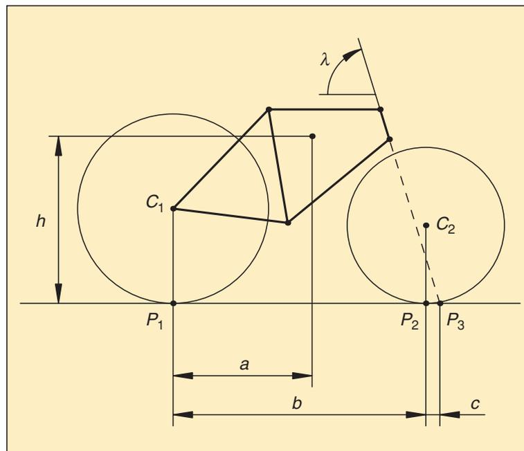
**Figure 1.** Parameters defining the bicycle geometry. The points  $P_1$  and  $P_2$  are the contact points of the wheels with the ground, the point  $P_3$  is the intersection of the steer axis with the horizontal plane,  $a$  is the distance from a vertical line through the center of mass to  $P_1$ ,  $b$  is the wheel base,  $c$  is the trail,  $h$  is the height of the center of mass, and  $\lambda$  is the head angle.
