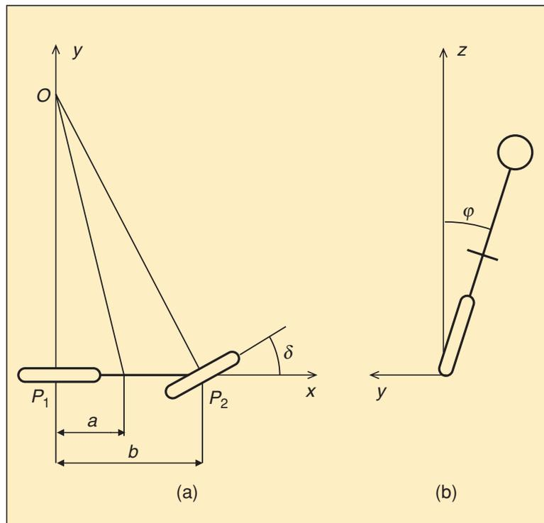
**Figure 3.** Schematic (a) top and (b) rear views of a naive ( $\lambda = 0$ ) bicycle. The steer angle is  $\delta$ , and the roll angle is  $\phi$ .
