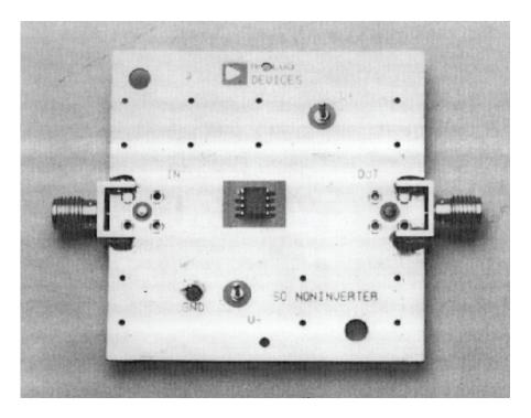
Fig. 12.30a: AD8001AR (SOIC) Evaluation Board—Top View
