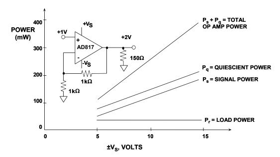
*Figure 12.76:* Power Dissipated in Video Op Amp Driver for Various Supply Voltages with Low Voltage Output Swing
