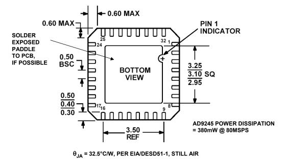
Figure 12.79: AD9245 CP-32 Lead-Frame Chip-Scale Package (LFCSP), Bottom View
