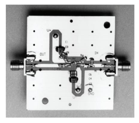
Fig. 12.30b: AD8001AR (SOIC) Evaluation Board—Bottom View
