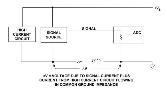
*Figure 12.8:* Any Current Flowing Through a Common Ground Impedance Can Cause Errors
