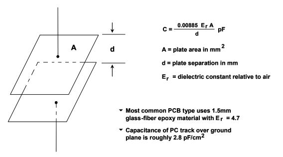
Figure 12.24: Capacitance of two parallel plates
