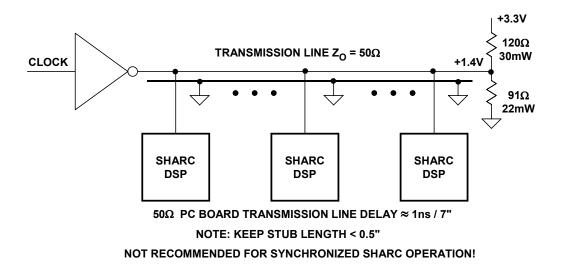
Figure 12.43: Clock Distribution Using End-of-Line Termination
