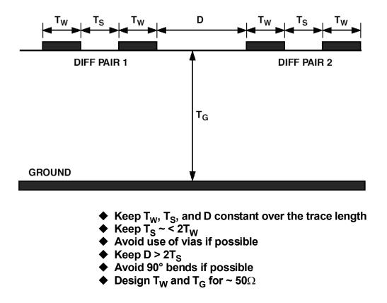
Figure 12.48: Microstrip PCB Layout for Two Pairs of LVDS Signals
