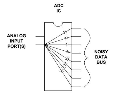
*Figure 12.28:* A High Speed ADC IC Using a CMOS Buffer/Latch at the Output Shows Enhanced Immunity of Digital Data Bus Noise
