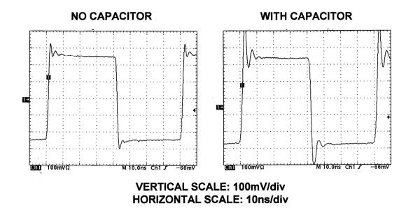
**Figure 12.31:** Effects of 10 pF Stray Capacitance on the Inverting Input on Amplifier (AD8001) Pulse Response
