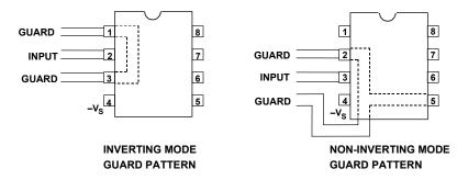
**Figure 12.16:** PCB Guard Patterns for Inverting and Noninverting Mode Op Amps Using Eight Pin SOIC (R) Package
