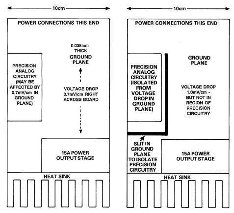
Figure 12.51: A Slit in the Ground Plane Can Reconfigure Current Flow for Better Accuracy
