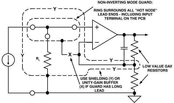
*Figure 12.14:* Noninverting Mode Guard Encloses all Op Amp Noninverting Input Connections Within a Low Impedance, Driven Guard Ring
