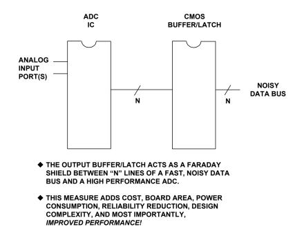
Figure 12.27: A High Speed ADC IC Sitting on a Fast Data Bus Couples Digital Noise into the Analog Port, thus Limiting Performance
