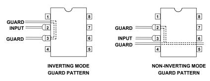
*Figure 12.15:* PCB Guard Patterns for Inverting and Noninverting Mode Op Amps Using Eight Pin MINI-DIP (N) Package
