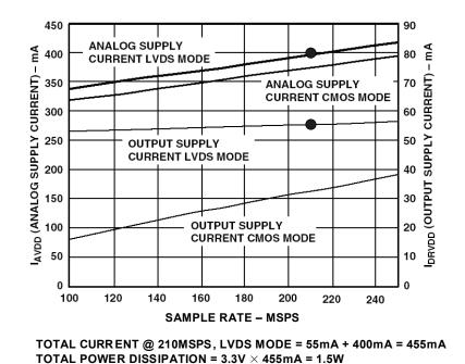
Figure 12.80: AD9430 12-Bit 170 MSPS/210 MSPS ADC Supply Current vs. Sample Rate for a 10.3 MHz Input
