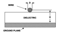
*Figure 12.35:* A Wire Microstrip Transmission Line With Defined Impedance is Formed by an Insulated Wire Spaced From a Ground Plane
