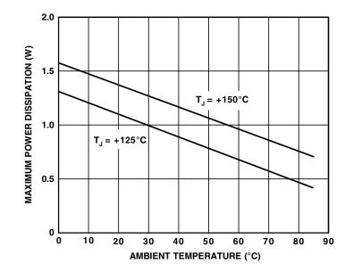
Figure 12.72: Thermal Rating Curves for AD8017AR Op Amp
