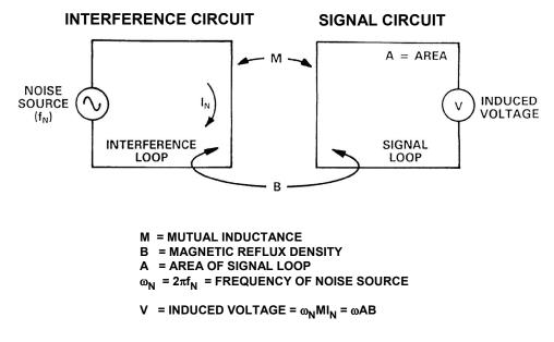
Figure 12.20: Basic Principles of Inductive Coupling
