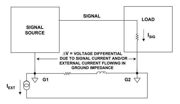
*Figure 12.7:* A More Realistic Source-to-Load Grounding System View Includes Consideration of the Impedance Between G1-G2, Plus the Effect of Any Nonsignal-Related Currents
