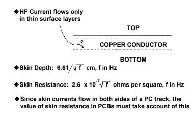
Figure 12.33: Skin Effect with PCB Conductor and Ground Plane
