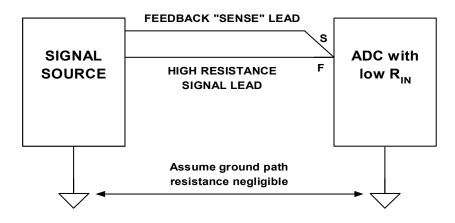
Figure 12.4: Use of a Sense Connection Moves Accuracy to the Load Point
