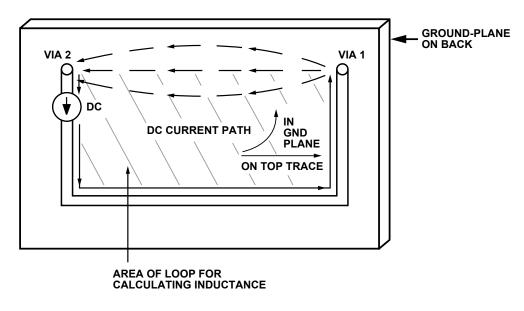
Figure 12.61: DC Current Flow for Figure 12.60
