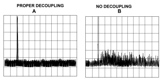
VERTICAL SCALES: 10dB/div, HORIZONTAL SCALES: 10MHz/div
