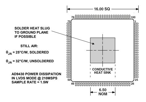
Figure 12.81: AD9430 100-Lead e-PAD TQFP
