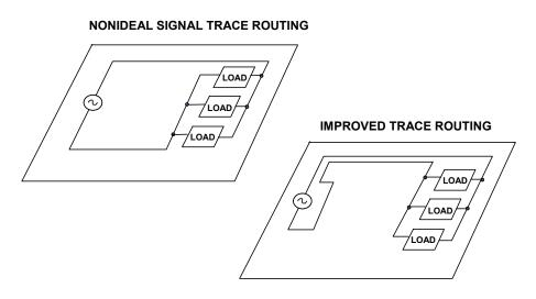
Figure 12.19: Nonideal and Improved Signal Trace Routing
