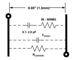
Figure 12.17: DA Plagues Dynamic Response of PCB-Based Circuits
