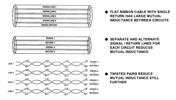
Figure 12.22: Mutual Inductance and Coupling Within Signal Cabling
