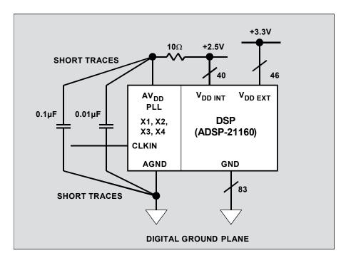
Figure 12.59: Grounding DSPs with Internal Phase-Locked-Loops (PLLs)
