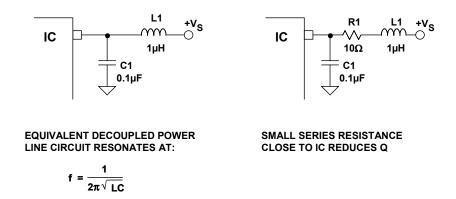
Figure 12.69: Resonant Circuit Formed by Power Line Decoupling
