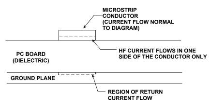
Figure 12.32: Skin Depth in a PCB Conductor
