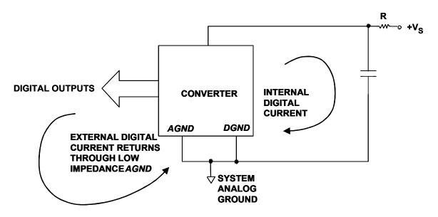
*Figure 12.49:* Analog (AGND) and Digital Ground (DGND) Pins of a Data Converter Should Be Returned to System Analog Ground
