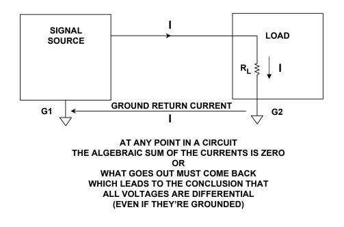
*Figure 12.5:* Kirchoff's Law Helps in Analyzing Voltage Drops Around a Complete Source/Load Coupled Circuit
