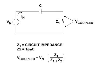
Figure 12.25: Capacitive Coupling Equivalent Circuit Model
