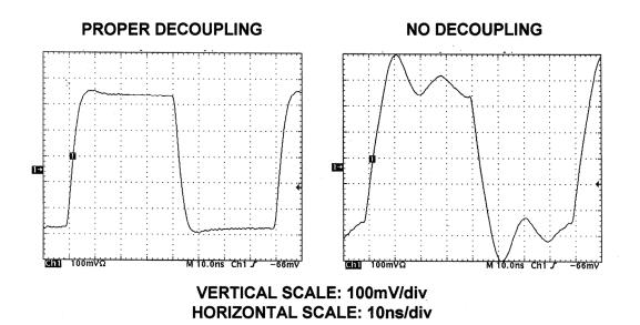
*Figure 12.68:* Effects of Inadequate Decoupling on the Phase Response of the AD9631 Op Amp
