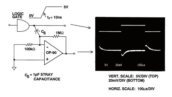
Figure 12.29 High Circuit Impedances Increase Susceptibility to Noise Pickup
