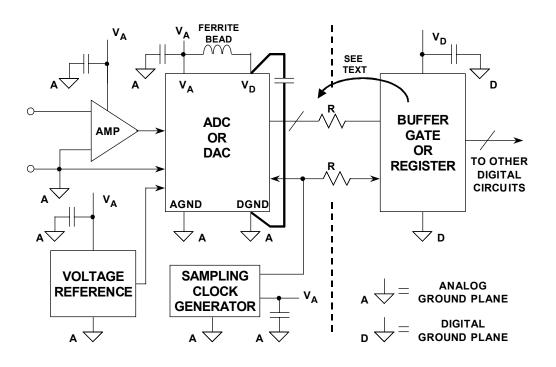
Figure 12.54: Grounding and Decoupling Points
