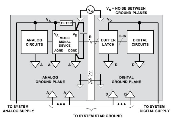
*Figure 12.57:* Grounding Mixed Signal ICs with Low Internal Digital Currents: Multiple PC Boards
