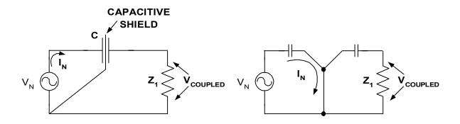
Figure 12.26: An Operational Model of a Faraday Shield
