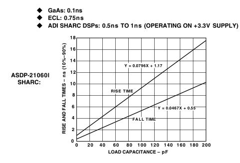
Figure 12.39: Typical DSP Output Rise Times and Fall Times
