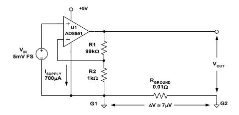
*Figure 12.10:* Unless Care Is Taken, Even Small Common Ground Currents Can Degrade Precision Amplifier Accuracy
