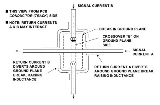
*Figure 12.64:* A Ground Plane Break Raises Circuit Inductance, and Increases Vulnerability to External Fields
