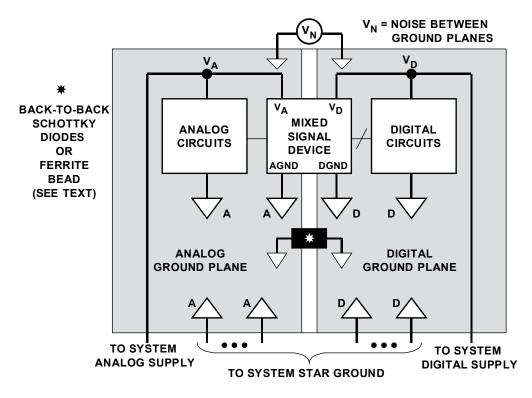
Figure 12.58: High Digital Currents: Multiple PC Boards
