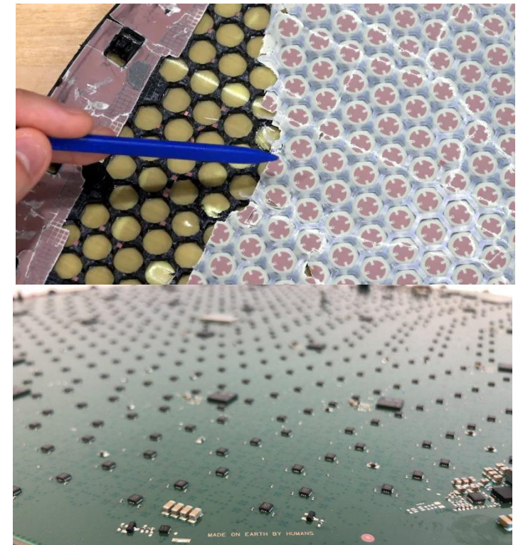
Inside a Starlink antenna (1280 elements)
