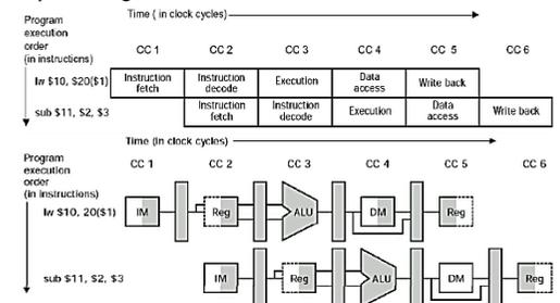
**Design of the pipelined control path:**
