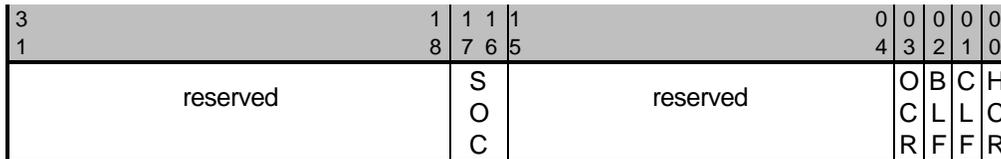
Figure 7-3: HcCommandStatus Register
