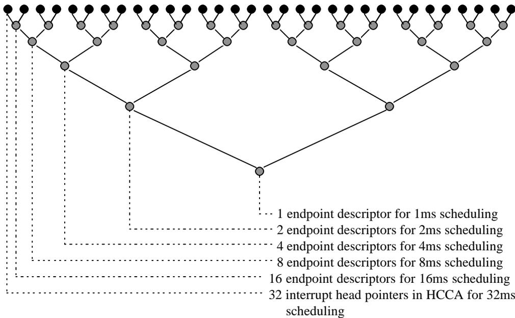
**Figure 5-4: Structure of Interrupt Lists**
