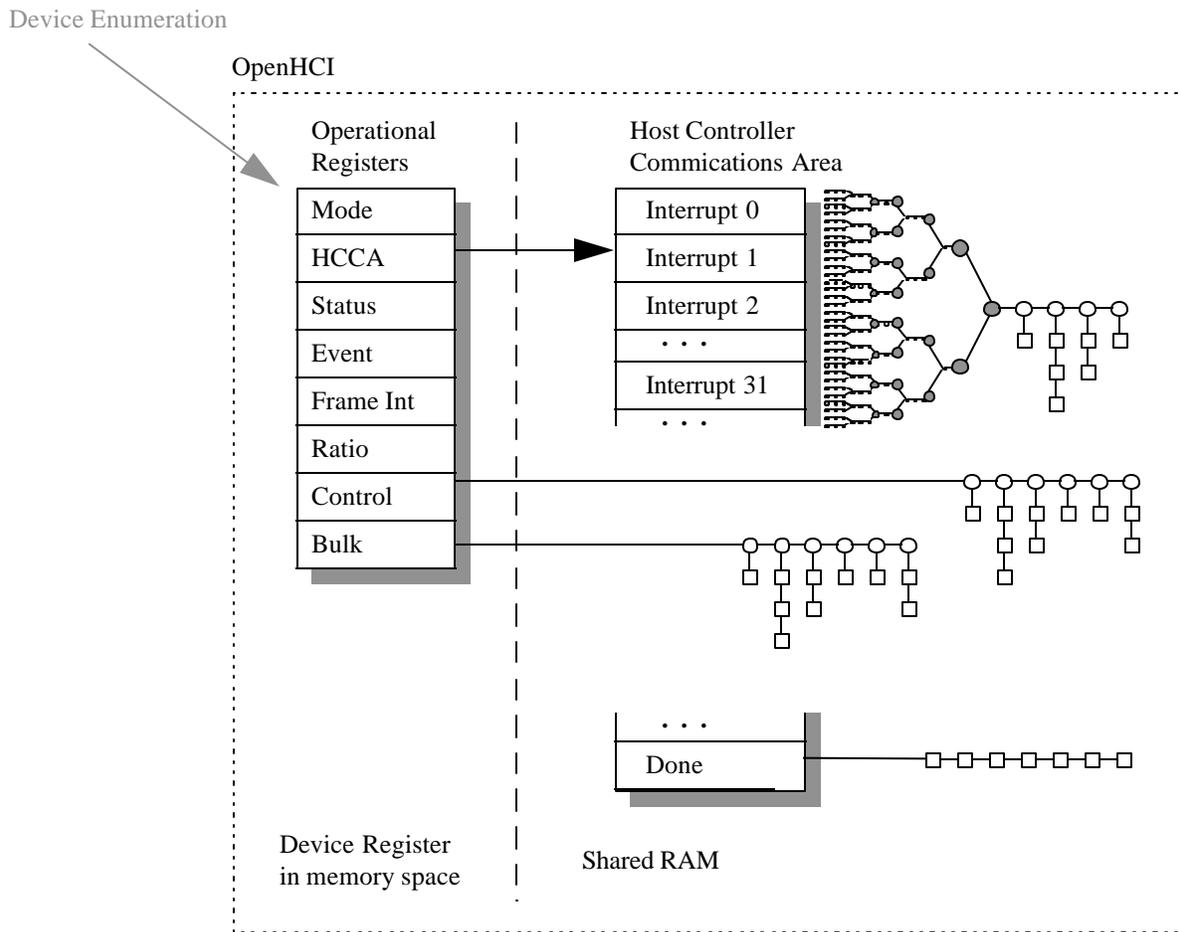
Figure 3-2: Communication Channels
