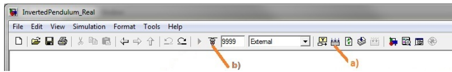
Figure 3.2: Press first a) to build the model, and then b) to connect to the target.
