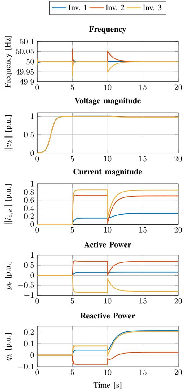
Fig. 3. The grid is black started then, at  $t = 5$  s the inverters are dispatched to the set-points of Table I and at  $t = 10$  s the transmission line connecting Inverters 2 and 3 is cut.
