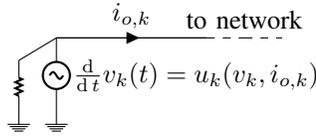
Fig. 1. Schematics of the decentralized control setup: the voltage  $v_k$  is fully controllable but only using local measurements.
