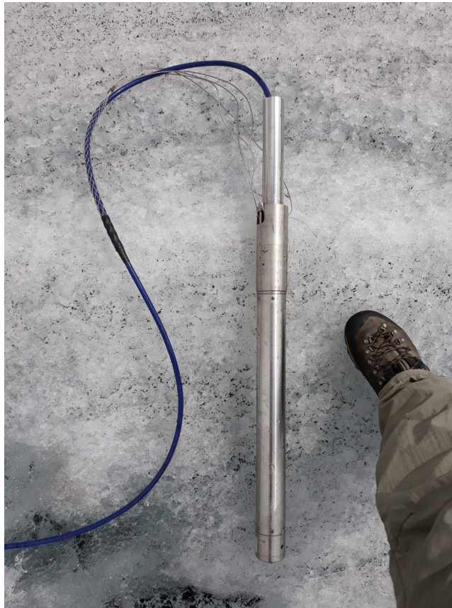
Figure 5: An example of the installed borehole seismometers. They were installed four meters into the ice. The blue cable is attached to the pelicase with the digitiser.
