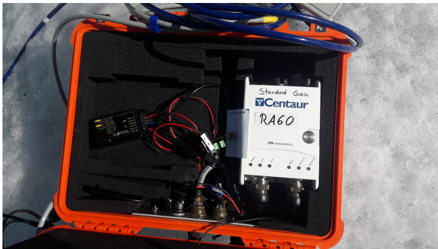
Figure 4: An example of content of the pelicase of a seismic station. The most important items are the digitiser (in this case a Nanometrics Centaur with standard gain), the battery and the GPS antenna.
