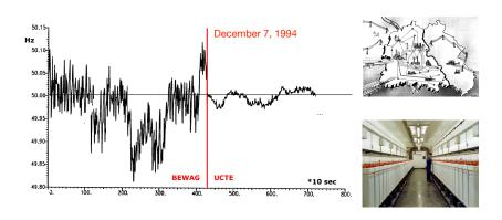
**before** re-connection: islanded operation based on **batteries** & boiler **afterwards** connected to European grid & **synchronous generation**
