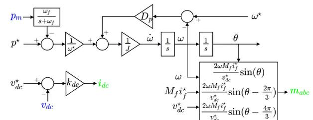
Figure 3. Synchronverter control diagram.
