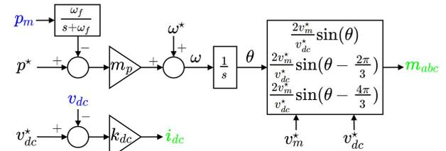
Figure 2. Droop control diagram.
