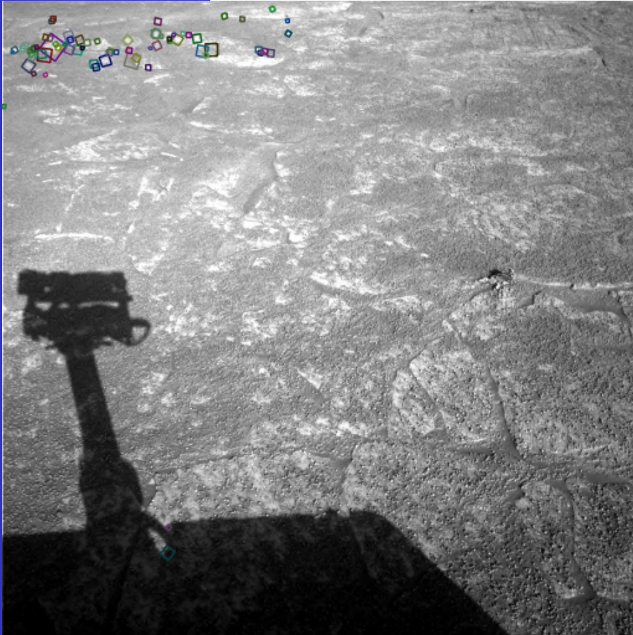
NASA Mars Rover images with SIFT feature matches Figure by Noah Snively
