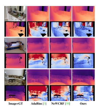
Figure 3. **Qualitative results on NYU.** Each pair of consecutive rows corresponds to one test sample. Each odd row shows the input RGB image and depth predictions for the selected methods. Each even row shows GT depth and the prediction errors of the selected methods clipped at 0.5 meters. The error color map is *coolwarm*: blue corresponds to lower error values and red to higher values.
