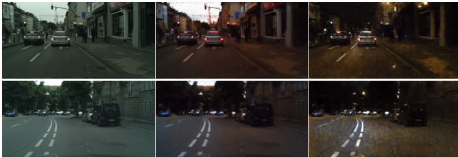
Fig. 9. Comparison of CycleGAN configurations for generation of synthetic stylized data from Cityscapes and Dark Zurich . From left to right: input Cityscapes image, stylized nighttime image with training on 256 \times 256 crops, stylized nighttime image with training on full 360 \times 720 images.
