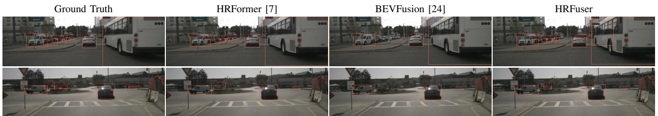
Fig. 13. Further qualitative detection results on nuScenes showing failure cases of HRFuser with 6 classes visualized: car, truck, bus, bicycle, motorcycle and pedestrian. From left to right: image with ground-truth annotation, prediction of HRFormer, 3D→2D projected predictions of BEVFusion, prediction of HRFuser. Best viewed on a screen at full zoom.
