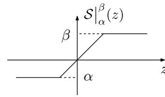
Fig. 2. Graphical representation of  $S_{\alpha}^{\beta(z)}(z)$ .
