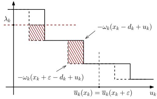
Fig. 4. Interpretation of the difference of the two integrals in (17) in the case of piecewise marginal value function, for  $\bar{u}_k(x_k) = \bar{u}_k(x_k + \varepsilon) = u_k^{\max} - d_k^{(f)}$ .
