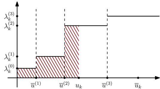
Fig. 5. Schematic representation of the piece-wise constant price curve that approximates the procurement cost in the presence of multiple sources. The shaded area corresponds to the total price paid to consume  $u_k$  at time  $k$ .
