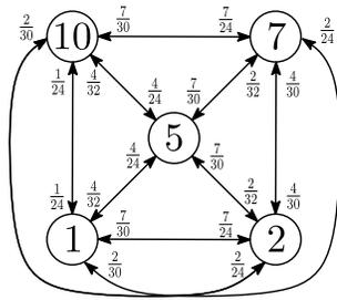
Fig. 8. Graph representation of the price process modeled as Markov process. The labels on the arrows are the corresponding transition probabilities from one price to another (transitions from one state to itself have been omitted).
