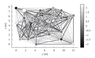
Figure 5. Network topology and node displacement for c-connectivity graph for c=0.1. Nodes' gray intensity represents the estimated offset  $\hat{o}_i$  after calibration. Black and gray edges represent the edges used for training and validation data sets, respectively.
