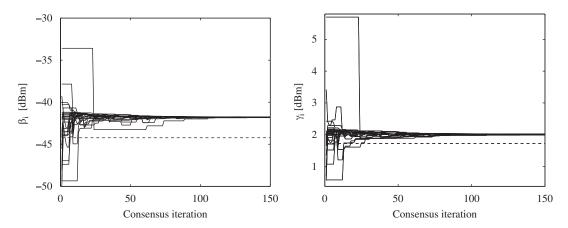
Figure 8. Convergence of parameter estimates  $\beta_i$ ,  $\gamma_i$  using randomized broadcast least-square consensus and consensus weight w = 0.5. The dashed lines are the centralized least squares estimates  $\hat{\beta}_{\text{LS}}$ ,  $\hat{\gamma}_{\text{LS}}$ .
