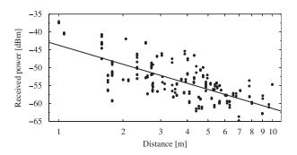
Figure 3. Estimated path-loss model for the wireless channel of the experimental environment using the standard centralized mean square estimate. The continuous line represents the path-loss function, while the dots are the measures experimentally collected.
