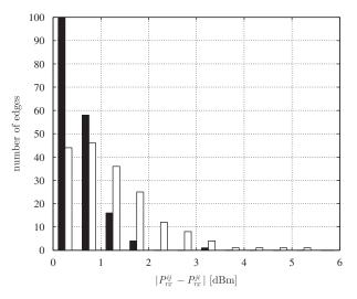
Figure 7. Asymmetric error distribution before  $(|\bar{P}_{rx}^{ij} - \bar{P}_{rx}^{ji}|, \text{ white})$  and after  $(|\bar{P}_{rx}^{ij} + \hat{o}_i - \bar{P}_{rx}^{ji} - \hat{o}_j|, \text{ black})$  distributed sensor calibration.
