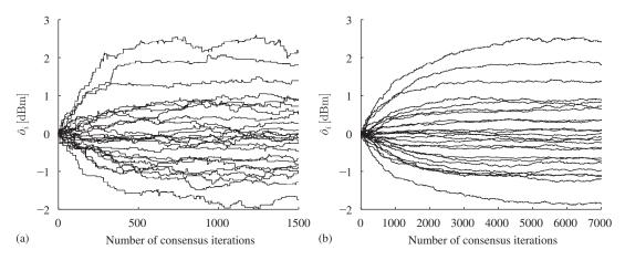
Figure 6. Offset estimation  $\hat{o}_i$  for each node of the considered WSN using randomized broadcast consensus for different values of the consensus weight w: (a) w = 0.05 and (b) w = 0.01.
