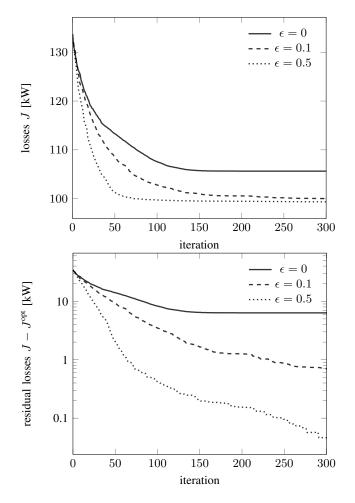
Fig. 3. Montecarlo analysis of the behavior of the algorithm for different values of  $\epsilon$ . As soon as  $\epsilon$  is greater than zero, the algorithm converges to the optimum. Also the rate of convergence depends on the choice of  $\epsilon$ . In this comparison we assume that one iteration corresponds to a complete iteration of the algorithm, regardless of how many hops are required for its completion.
