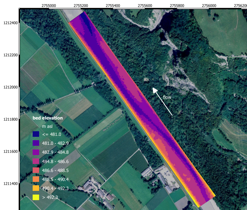
Figure 8.1 Planar view of the initial bottom elevation of the Alpine Rhine river
